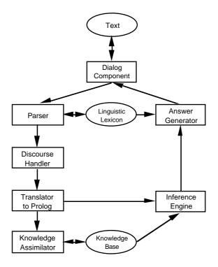
The *Discourse Handler* analyses and resolves inter-text references and updates the discourse representation structures generated by the parser. Optionally, the *Translator*
