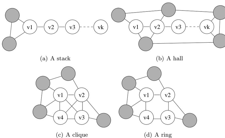
Figure 2: Examples of the four different subgraph structures.
