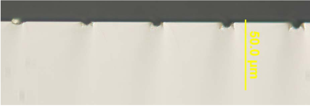
Figure 3.38 Laser features machined in lithium niobate with 1-5 passes, 1μJ pulses at 1kHz, with a 100mm/min feedrate.
