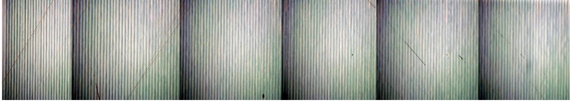
Figure 5.8 Domains across a 10 mm section of laser direct write fabricated PPLN with a 40 \mu\text{m} period.
