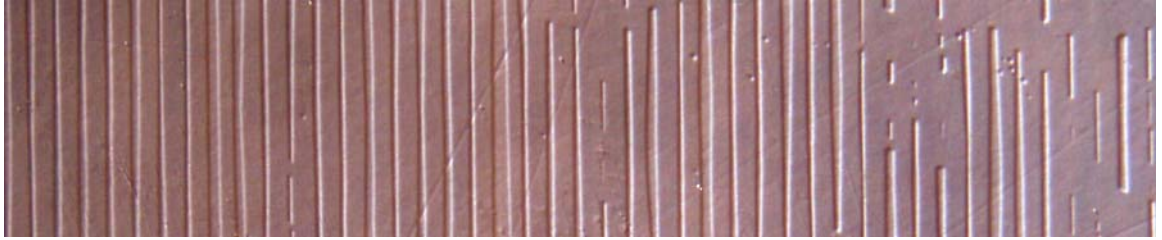
Figure 2.37 Example of PPLN with good periodicity but with some duty cycle errors and missing inversions in some regions.
