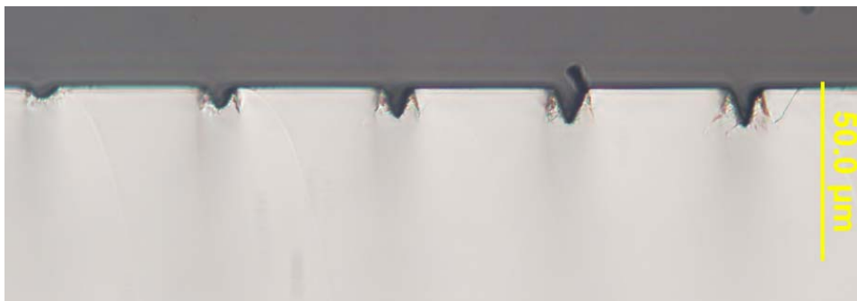
Figure 3.37 Laser features machined in lithium niobate with 1-5 passes, 1 \mu\text{J} pulses at 1kHz, with a 25mm/min feedrate.
