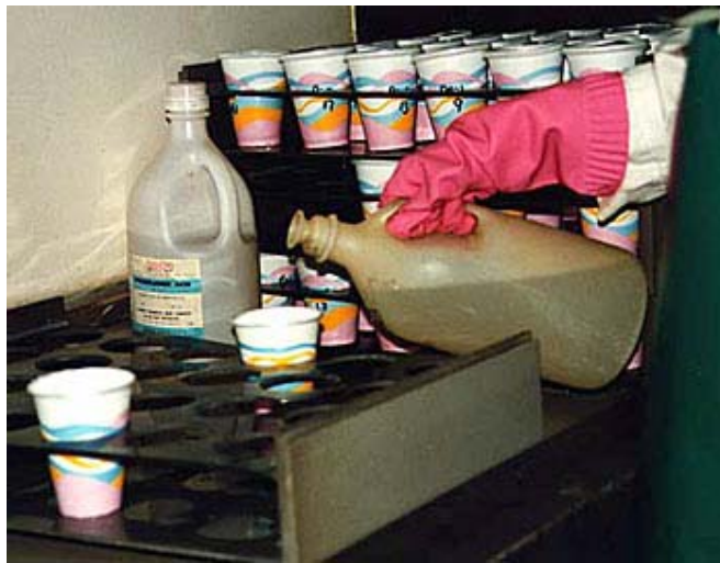
Above: The laboratory personnel may have minimised the likelihood of a spill through the introduction of cup supports for the digestion cups.
