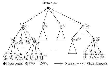
Figure 6 4-branch Dispatch Tree of Model Tm<sup>+</sup> with 64 Mobile Agents
