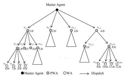
Figure 5 4-branch Dispatch Tree of Model Tm with 64 Mobile Agents
